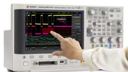
Figure 2. The industry's first 8.5" capacitive touch display with large, touchable targets.
