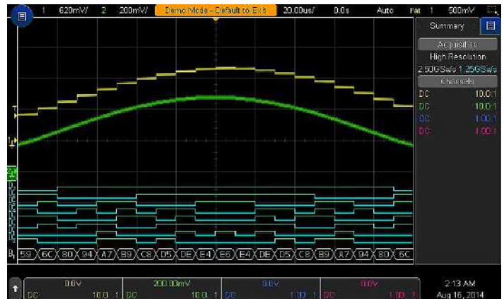
Figure 24. Optional digital channels allow a timing view of up to 16 channels. Tightly integrated, they work with the analog triggers and serial triggers/decoding.
