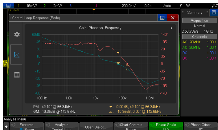
Figure 30b. New control loop response analysis (bode plot) shows the gain/phase plot over frequency sweep.
