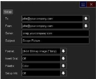
Figure 6. With the optional LAN/ VGA module you can email yourself setups, data and screenshots.
